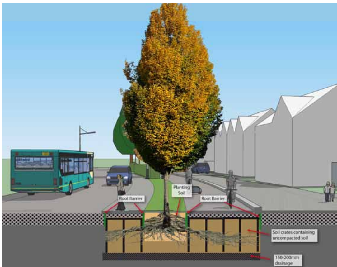
41. Plans and sections should demonstrate how tree crown and root growth will be accommodated in relevant growing areas.
