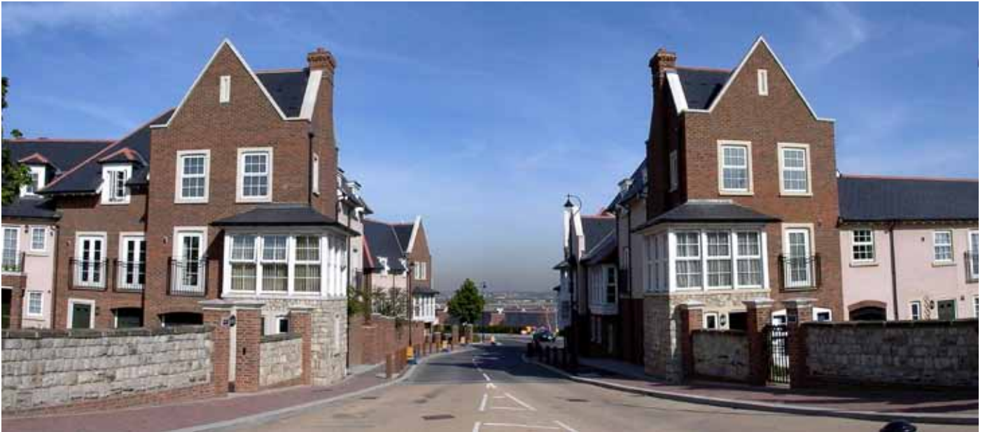
33. Buildings on significant corners should be designed to have a degree of prominence, whilst also having a plan and facade that offer a frontage treatment when seen from either street. Ingress Park, Greenhithe.
