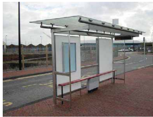
Cantilevered shelter Style 1
