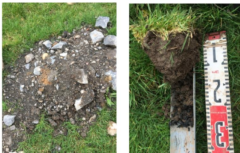
**Figure 1:** Left – Made ground with large amounts of demolition rubble; Right – Topsoil over asphalt at 25 cm depth
